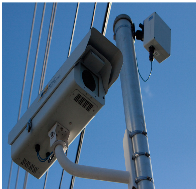
One of the nine red light cameras monitors traffic lights in Lakeland.
